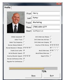
The Profile Form has more loops than the L.A. Interstate. I labeled each CheckBox with a 3 digit number at the end. The first two numbers represent the digit in the 18-digit code for the user. The last number represents the value of each CheckBox, the fifth resume reviewed will place a five for the fifth digit in the progress code. (See Code Below)
